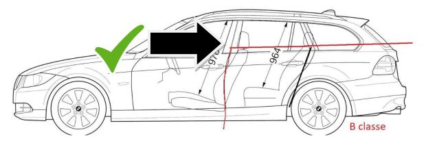
In the sketch the backseat is very high, just to give you an impression. As long as the backseat is original. When checking to see if the enclosure is valid for B / R Unlimited you must use a line parallel to the ground as shown above, the two examples below although they are exaggerated are both wrong.
