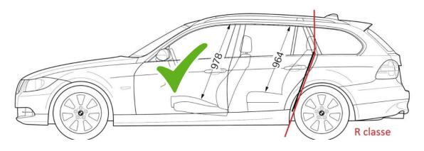
The diagram below shows a car that would not be allowed in R as the enclosure encroaches on the passenger cabin.
