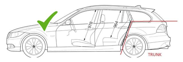
When checking to see if the enclosure is in the trunk you must use a line parallel to the ground, the example below although exaggerated is wrong.
