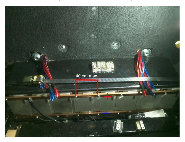
In this picture the metal bar is in total bigger than 40 cm.
